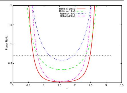
**Figure 1.** Power in  $k \neq 0$  sidebands relative to power in k = 0 sideband for challenge source 1B.3.2. The true parameters were  $\lambda = 1.44$ ,  $\kappa = 1.295$ . Our estimated inclination was  $\kappa = 1.262$ .
